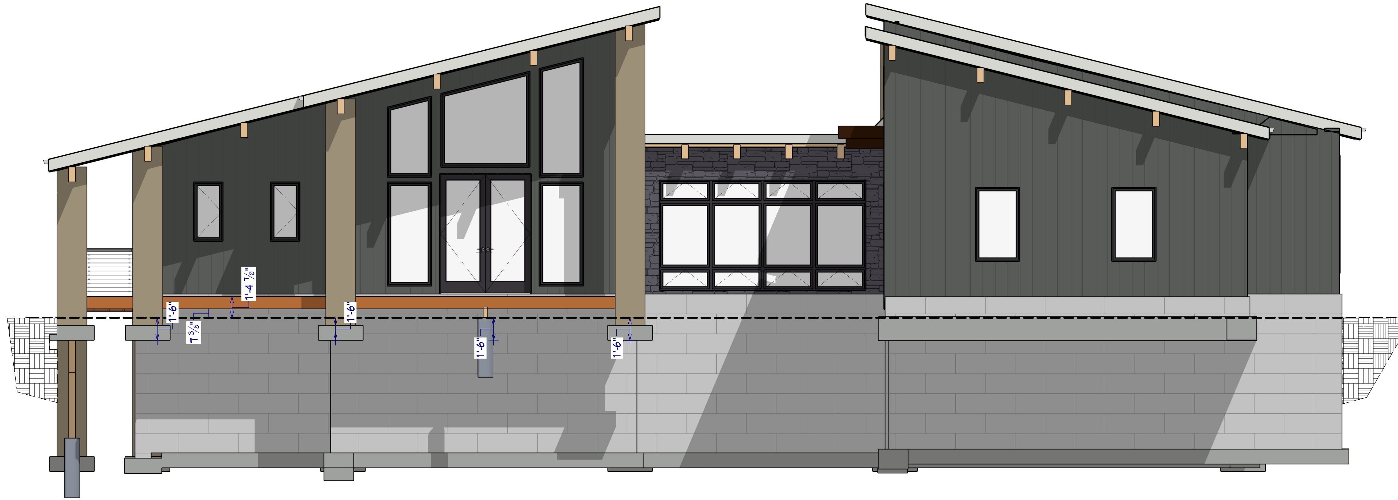
E1 FRONT (SOUTH) ELEVATION 1/4 IN = 1 FT
